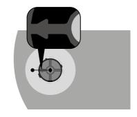
Insert Bracket ① into the hole from the inside of the mask. Look for the arrow sign on the bracket. Ensure the arrow faces and aligns with the red dot located on the outside of the mask.
