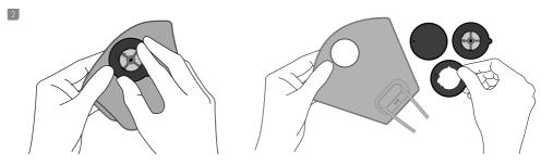
Detach the bracket from the mask to remove all remaining air valve components.
