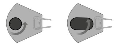
To remove the air valve or the fan unit\*, detach by rotating counterclockwise.
