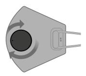
Align the dots on Bracket ② and Air Valve Cover in a linear position. Spin the Air Valve cover clockwise.
