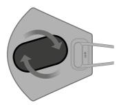
Align the dots on Bracket  ${\Large @}$  and the Fan Unit in a linear fashion. Spin the Fan Unit clockwise.
