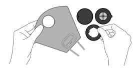
Remove all air valve components. Refer to: "How to Remove the Air Valve"
