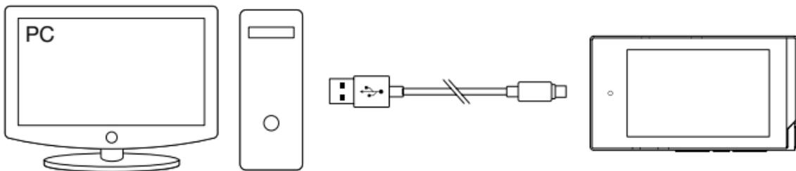
1. Micro USB cable connects the PC and Micro USB port.
