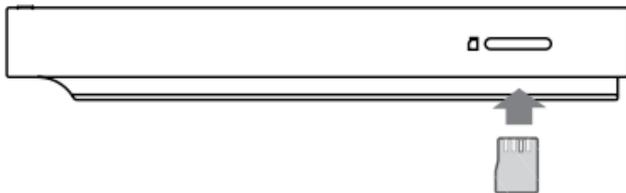
1. Properly place the microSD Card in the microSD card slot as shown in the picture. Gently press the card to insert it.
